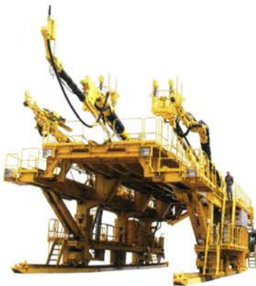
Tunnel Work Station (TWS) Self-propelling 2-boom with concrete sprayer
