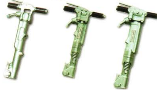
Hand drill For downward drilling in quarries, road construction.
